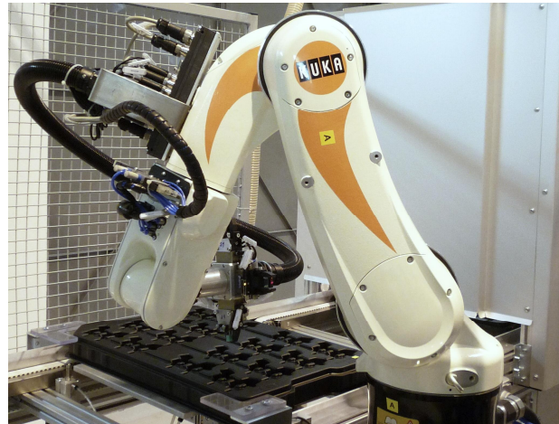
Robot A – manipulation with parts in loading palette
