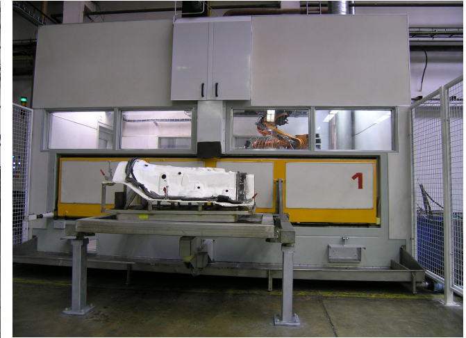
ABB cabin after reconstruction with KUKA robot
