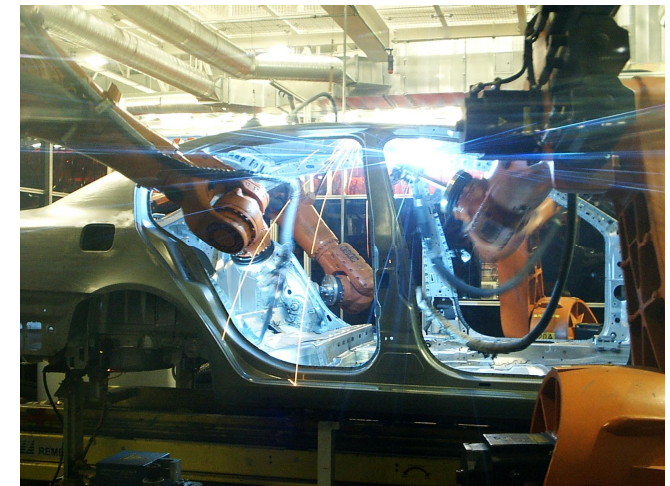
AFO 210 – robotic welding MIG
