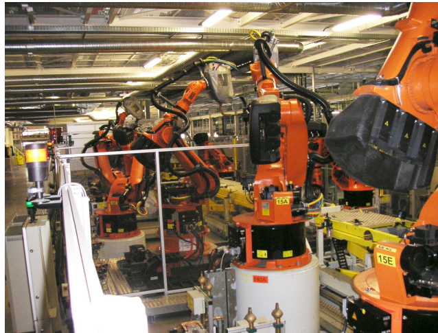
AFO 140-160 – robotic afterwelding
