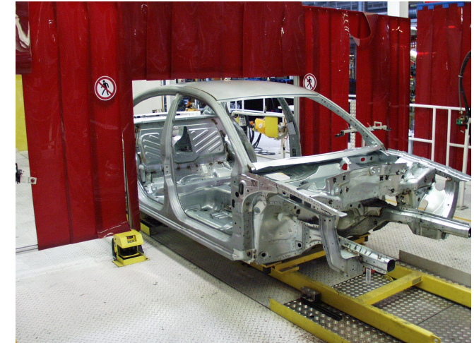
AFO 230 – handy final welding MIG
